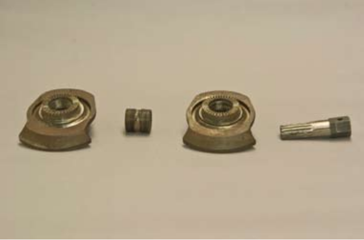
Two crank webs are joined by a hollow screw with a thread at each end with different pitches. The screw is turned a fraction of a turn with each grab by the special splined driver shown at the right. This special tool was made by Rainer.
