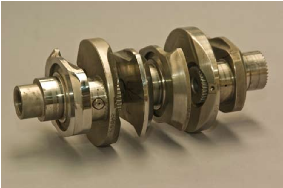
The top photograph is a complete HIRTH crank assembly. It is made up of pieces joined by special screws and matched serrations.
