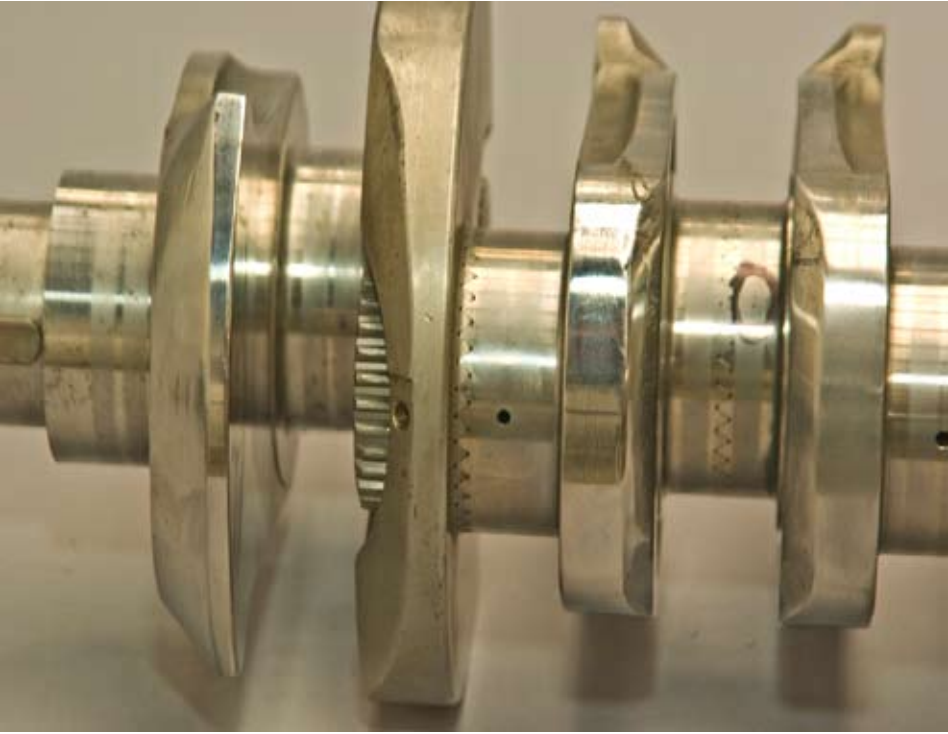
Two crank webs are joined by a hollow screw with a thread at each end with different pitches. The screw is turned a fraction of a turn with each grab by the special splined driver shown at the right. This special tool was made by Rainer.
