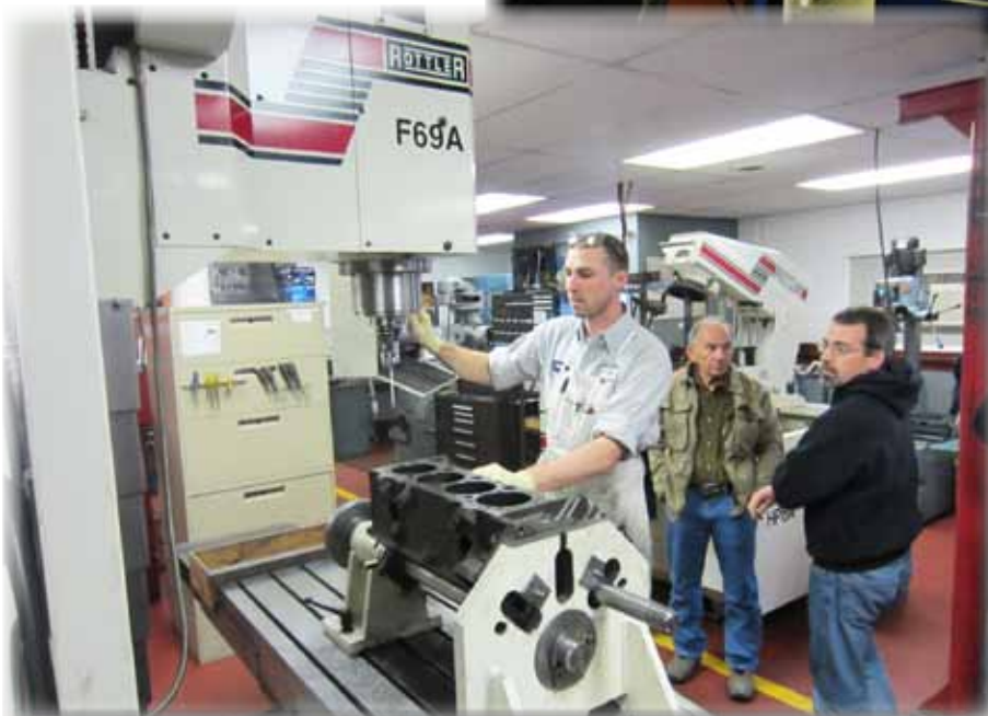
Nathan explained and demonstrated engine blueprinting, precision measuring and cylinder boring techniques on the Rottler F69A CNC Machining Center.
