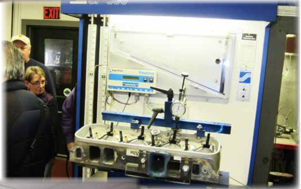
The R&L Superflow SF600 flow bench.
