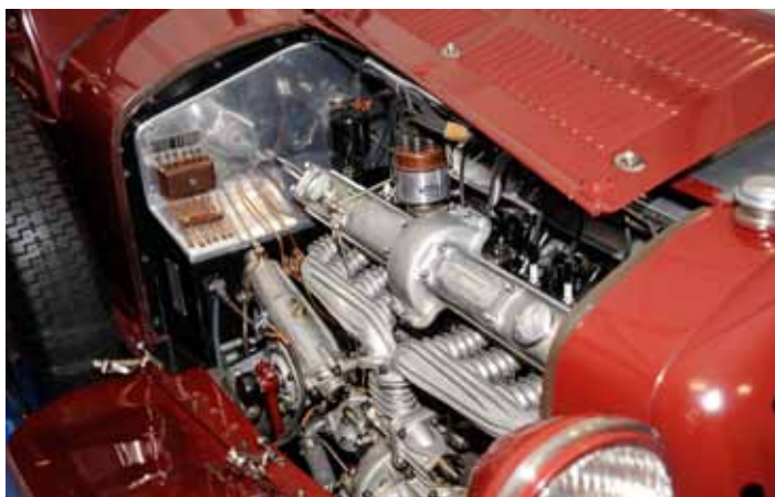
A pre war Alfa...this is a version of the car Enzo Ferrari drove in races. Note the center drive to the cam shafts. Wonderful, beautiful engineering.
