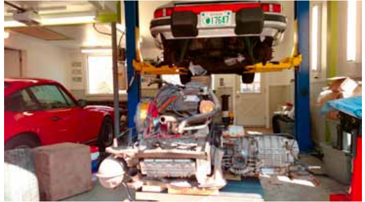
Jim dropped the engine in the Targa for some oil fixes and "while you're in there repairs"
